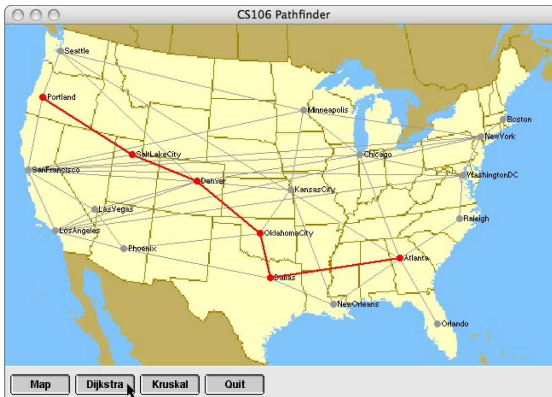
Figure 2. Result of applying Dijkstra’s algorithm to connect Portland and Atlanta
